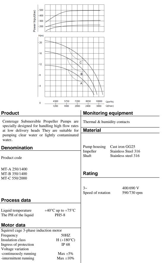
Voltage imbalance between phases max 2% No. of start/hour max 3
